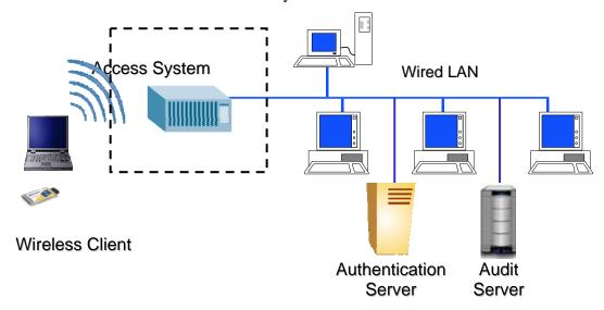
Figure 4: Example WLAN Access System with Authentication and Audit Servers
