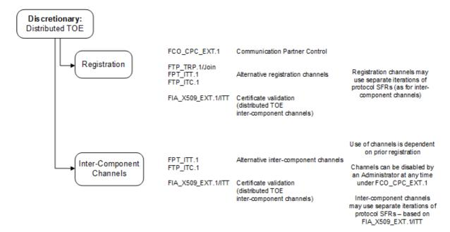
Figure 19: Distributed TOE SFR Architecture
