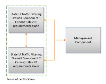
Figure 4: Distributed TOE use case with Management Component out of scope
