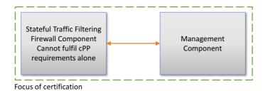
Figure 5: Management Component required to fulfil cPP requirements
