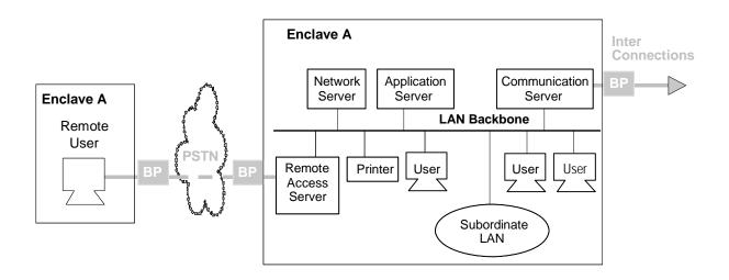
Boundary Protection (e.g., Firewall, Guard, Virtual Private Network, In-line Encryptor)
