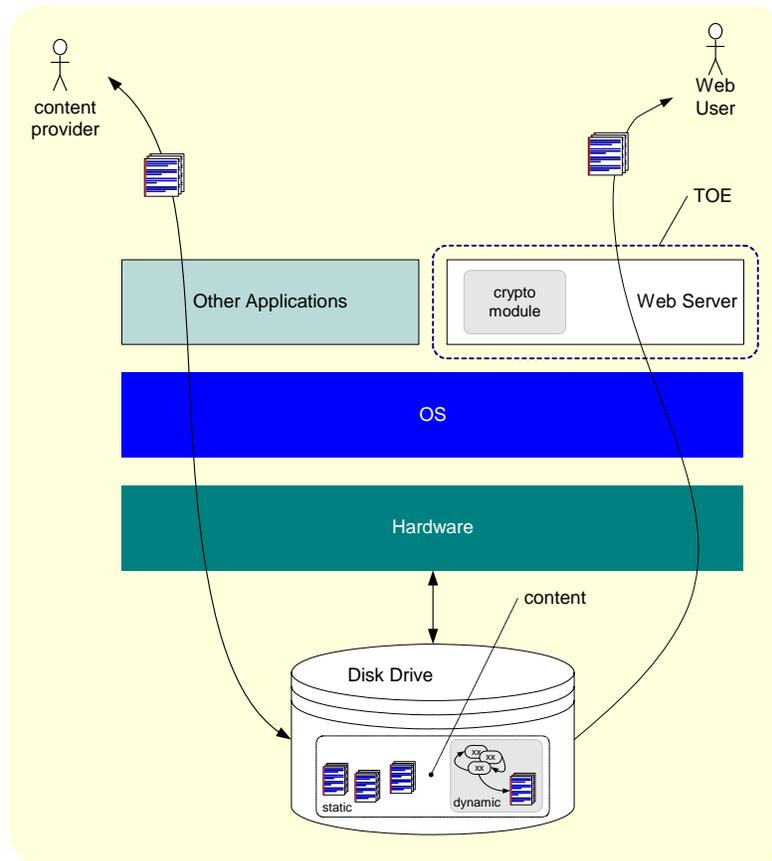
**Figure 2-2: The TOE and its execution environment**
