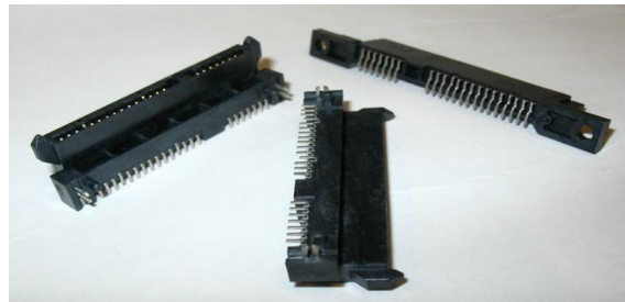
Figure 8: SATA connectors with separate pins
