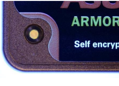
Figure 11: Screw head in UV light
