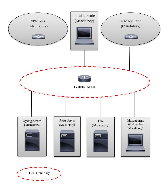
Figure 1 TOE Example Deployment for Cat8200, Cat8500
