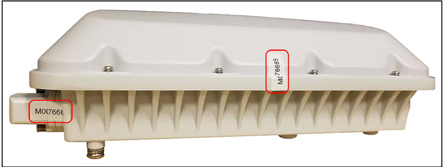
FIGURE 278 T610 AP Side Seal Detail
