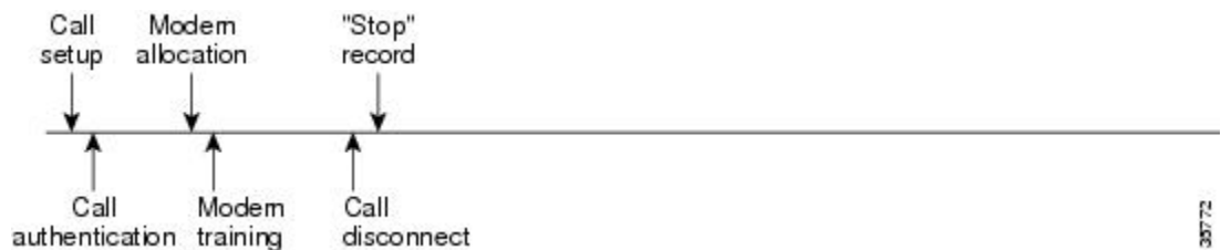
Figure 6: Modem Dial-In Call Setup Sequence With Call Disconnect Occurring Before User Authentication and With Resource Failure Stop Accounting Enabled
