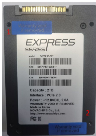
Figure 27. U.2 Enclosure and Tamper-evident label locations
