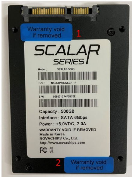
Figure 26. 2.5inch SATA and R-SATA Enclosure and Tamper-evident label locations
