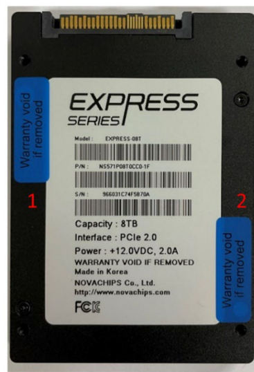
Figure 27. U.2 Enclosure and Tamper-evident label locations
