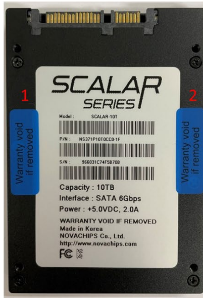
Figure 26. 2.5inch SATA and R-SATA Enclosure and Tamper-evident label locations
