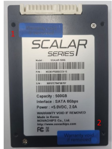
Figure 26. 2.5inch SATA and R-SATA Enclosure and Tamper-evident label locations
