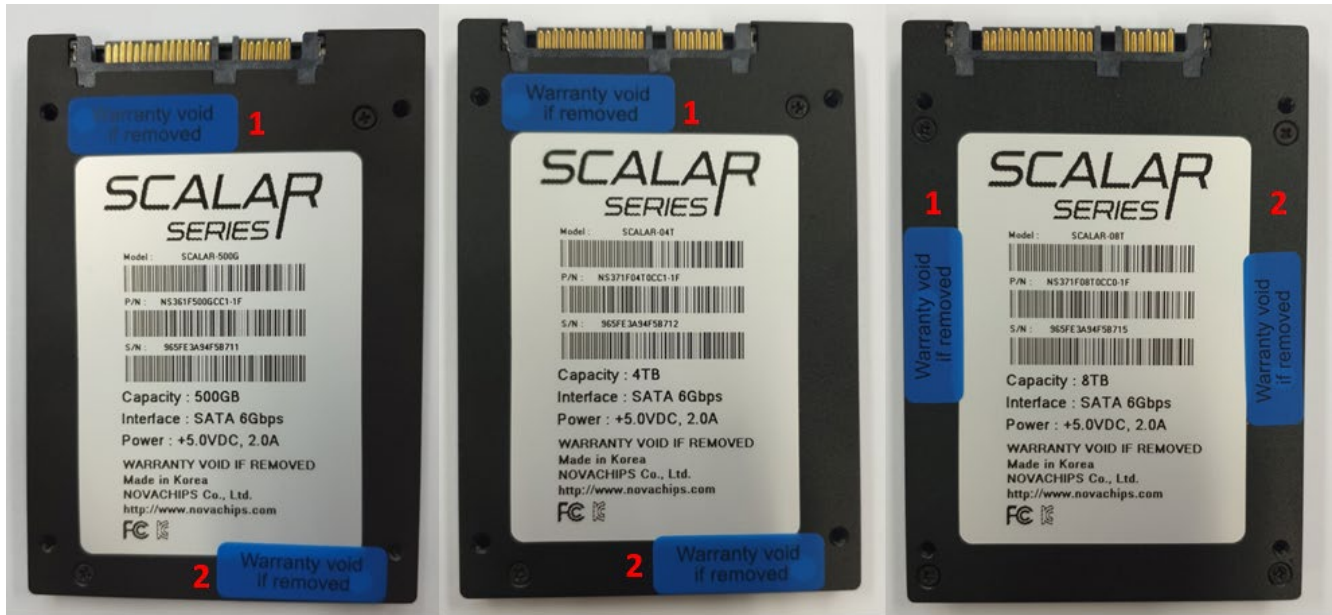
Figure 22. Enclosure and Tamper-evident label locations
