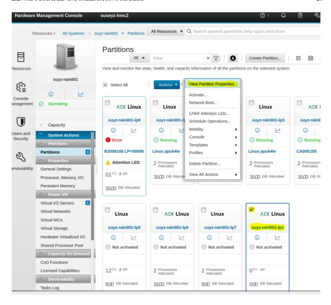
Now select "Virtual Storage" in the menu on the left and add a logical volume. Provide a device name and the storage size to be allocated.
