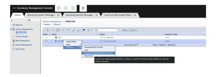
Now enter the FTP credentials including host name and filepath. In the next step select the [...]/suse.ins (not [...]/susehmc.ins) and proceed. After providing the password for the user the image will be loaded and should succeed without any problems.
