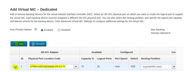
Finish setting up the virtual NIC by approving with OK. The next step is to mount the iso image to the virtual optical device. Therefore, select "Virtual Storage" in the menu on the left and the "Virtual Optical Device" tab. Now add a virtual optical device by providing the device name and selecting the virtual I/O server. After continuing with OK select "Action" > "Load" in the "Virtual Optical Device" tab and choose the SUSE Linux Enterprise 15 SP4 iso image.
