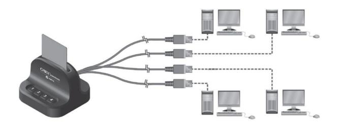
Figure 1 – Multi-Domain Smart Card Reader Evaluated Configuration
