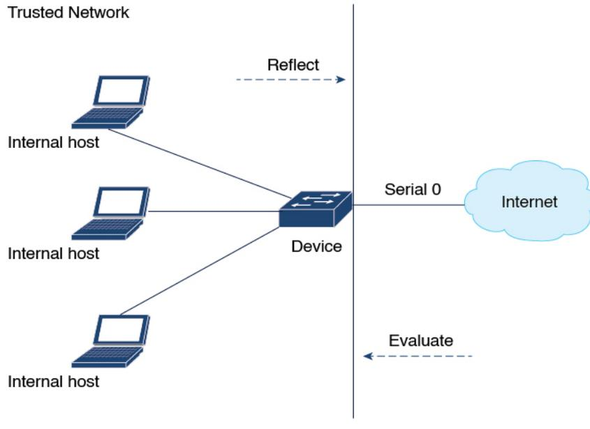
In the second topology, reflexive access lists are configured for the internal interface. This allows external traffic to access the services in the Demilitarized Zone (DMZ), such as DNS services. But, prevents IP traffic from entering your internal network - unless the traffic is part of a session already established from within the internal network.
