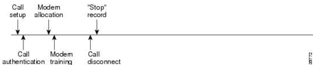
The figure below illustrates a call setup sequence with call disconnect occurring before user authentication and without AAA resource failure stop accounting enabled.
