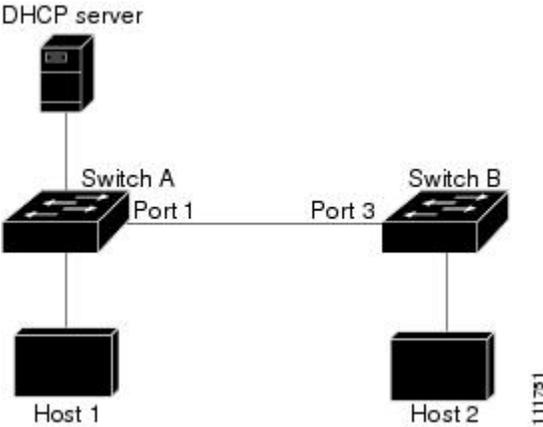
Configuring interfaces to be trusted when they are actually untrusted leaves a security hole in the network. If Switch A is not running dynamic ARP inspection, Host 1 can easily poison the ARP cache of Switch B (and Host 2, if the link between the switches is configured as trusted). This condition can occur even though Switch B is running dynamic ARP inspection.
