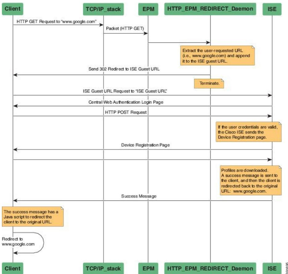
1. A user accesses a network for the first time and sends an HTTP request to access [www.google.com](http://www.google.com). When the user first accesses the network, a MAC authentication bypass (MAB) is triggered and the MAC address is sent to the Cisco ISE.
