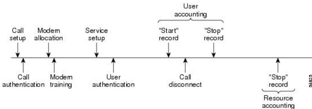
The figure below illustrates a call setup sequence with call disconnect occurring before user authentication and with AAA resource failure stop accounting enabled.
