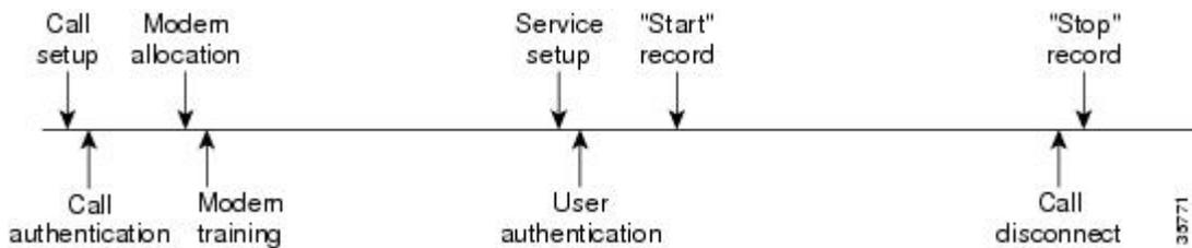
The figure below illustrates a call setup sequence with normal call flow (no disconnect) and with AAA resource failure stop accounting enabled.
