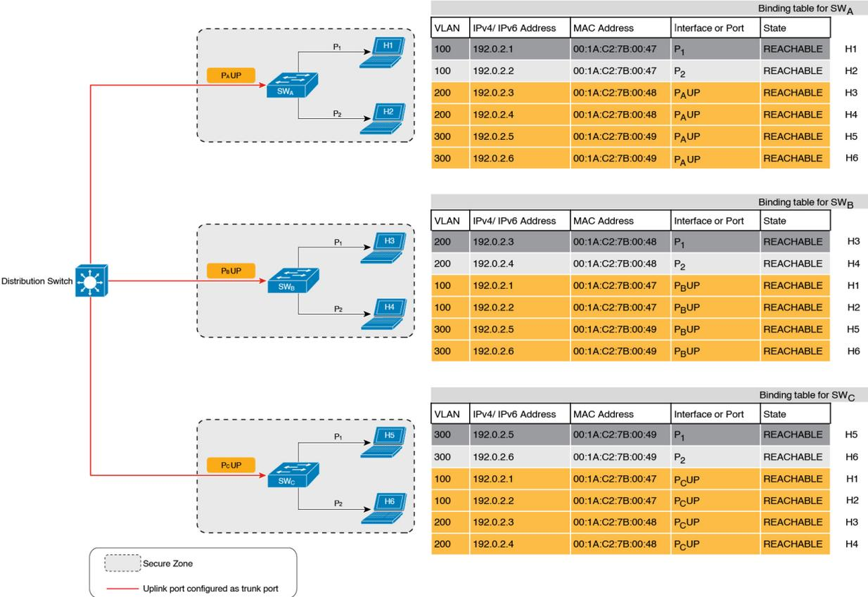
Figure 35: Secure Zone 2 - Efficient and Scalable Secure Zone When Binding Tables are Decentralized
