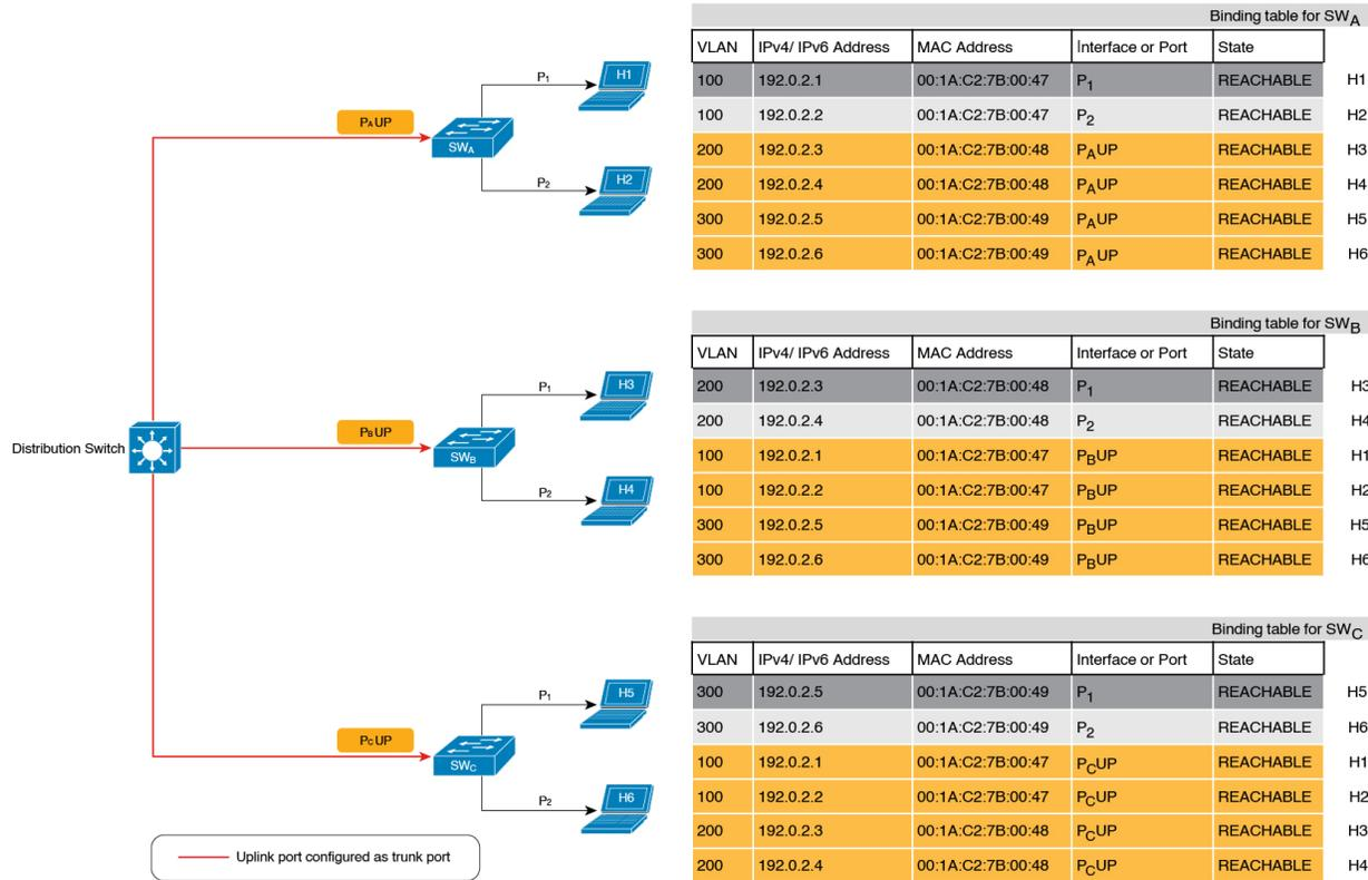
By contrast see figure #unique\_753 unique\_753\_Connect\_42\_fig\_obz\_xwj\_srb below. Here when SW<sub>A</sub> intercepts the packet of a host that is not attached to it (say H3 which is directly attached to SW<sub>B</sub>), it does not create an entry because it detects that H3 is attached to a device that is configured as a switch (**device-role switch** option) and the uplink port of the switch (where the packet came from) is a trusted port (**trusted-port** option).
